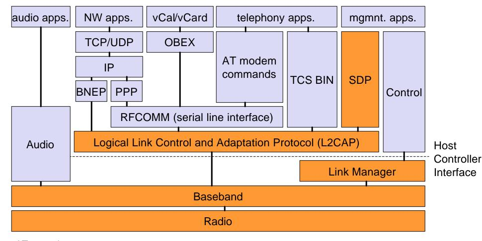
AT: attention sequence OBEX: object exchange TCS BIN: telephony control protocol specification – binary BNEP: Bluetooth network encapsulation protocol
