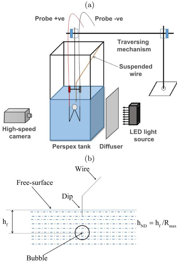
FIG. 1: (a) Schematic of the experimental set-up, and (b) illustration of various physical parameters.
