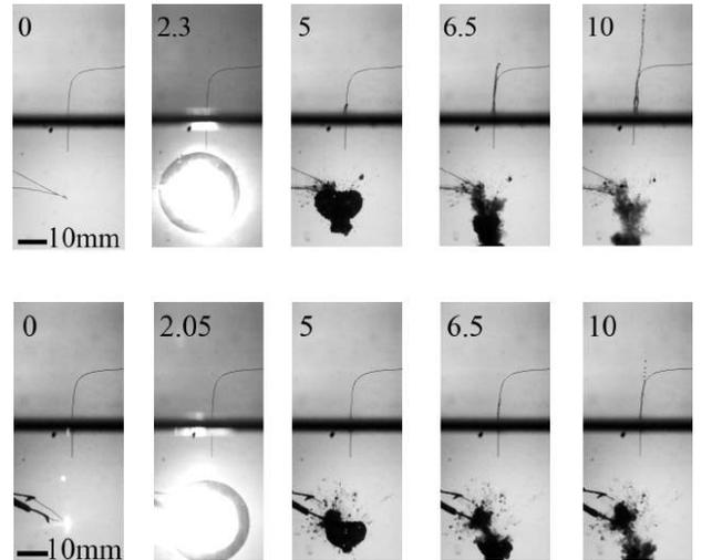
FIG. 4: Effect of  $h_{ND} \equiv (h/R_{max})$  on the bubble interactions and microjets.  $h_{ND} = 1.6$  (top row) and  $h_{ND} = 2.1$  (bottom row) for  $R_{max} = 12.2$  mm. The numbers in each image represent times in ms.
