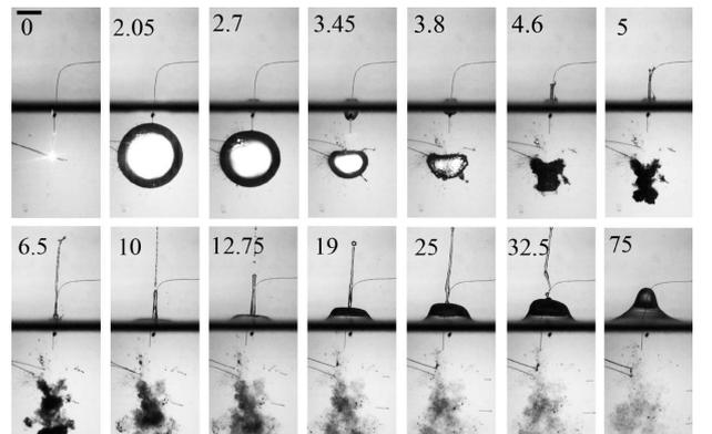
FIG. 2: Illustration of bubble dynamics and free surface microjets. Here,  $R_{max} = 12 \text{ mm}$  and  $h_{ND} = 1.3$ . The number in each image represents the time in ms.
