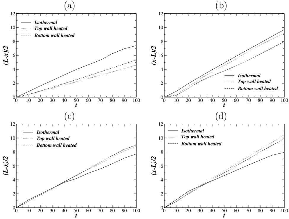
Figure 4: The distance travelled by the lighter, (a,c), and heavier (b,d) fronts, respectively. The panels (a,b) and (c,d) correspond to  $Re = 100$  and  $Re = 1000$ , respectively. The rest of the parameter values are the same as those used to generate Fig. 3.
