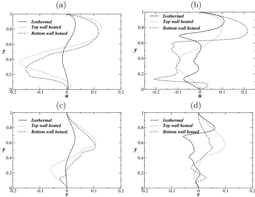
Figure 5: The axial ( $u$ ) and the wall-normal ( $v$ ) velocity profiles at the tip of the heavier fluid at (a,c)  $t = 40$  and (b,d)  $t = 100$ , respectively for  $Re = 1000$ . The rest of the parameter values are the same as those used to generate Fig. 3.
