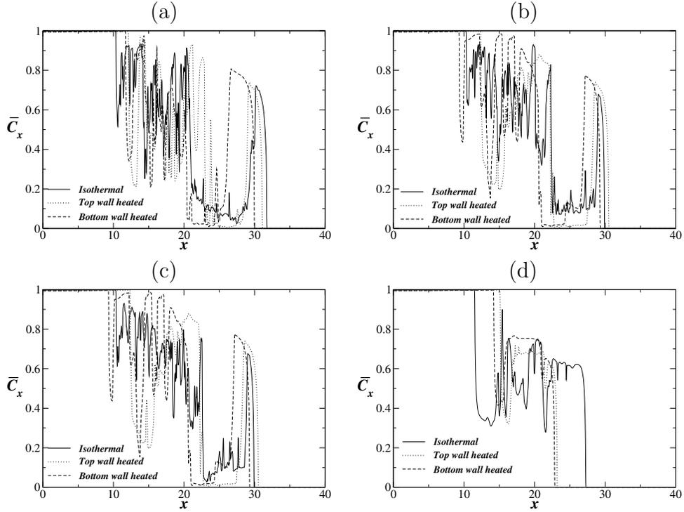
Figure 10: Variation of the transverse averaged volume fraction of the lighter fluid,  $\bar{C}_x$  in the axial direction at  $t = 100$  for (a)  $\mu_r = 0.01$ , (b)  $\mu_r = 0.1$ , (c)  $\mu_r = 1$ , (d)  $\mu_r = 10$ . The rest of the parameter values are the same as those used to generate Fig. 9.
