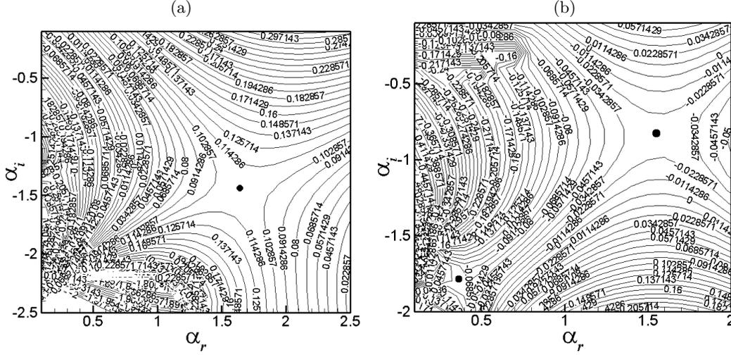
FIGURE 18. Isocontours of  $\omega_i$  in the complex wavenumber plane for (a) The unstratified case,  $R_s = 0$ . At the saddle point (filled circle),  $\omega_{0i} = 0.108$ . (b)  $R_s = 1$ .  $\omega_{0i} = -0.026$  and  $-0.071$  at the top and bottom saddle points (shown by filled circles), respectively. The values of the rest of the parameters are  $\text{Re} = 100$ ,  $R_t = 2$ ,  $h = 0.5693$ ,  $q = 0.1138$ .
