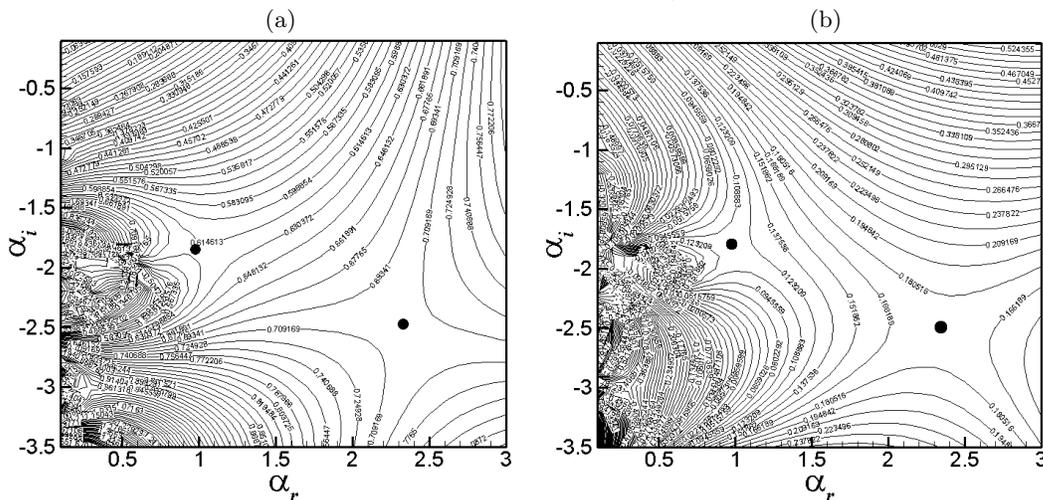
FIGURE 17. Isocontours of (a)  $\omega_r$  and (b)  $\omega_i$  in the complex wavenumber plane. The parameters are  $\text{Re} = 100$ ,  $R_s = -1$ ,  $R_t = 2$ ,  $h = 0.5693$ ,  $q = 0.1138$ . The value of the complex frequency  $\omega_0$  at the top and bottom saddle points (shown by filled circles) are  $0.616 + 0.118i$  and  $0.706 + 0.174i$  respectively.
