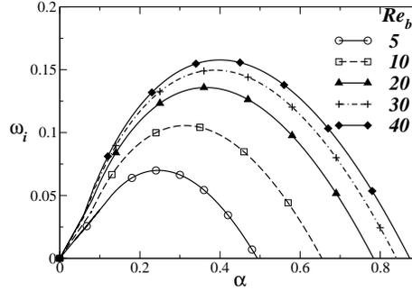
FIGURE 5. Comparison with the dispersion curves ( $\omega_i$  versus  $\alpha$ ) of Betchov & Szewczyk (1963) (symbols) for different values of  $Re_b$  with present results (lines). Here velocity profile given by  $U = U_0 \tanh(y/\delta)$  is used as suggested by Betchov & Szewczyk (1963), and  $Re_b$  is defined as  $U_0 \delta \rho / \mu$ . Note  $Re_b$  is defined differently from  $Re$ .
