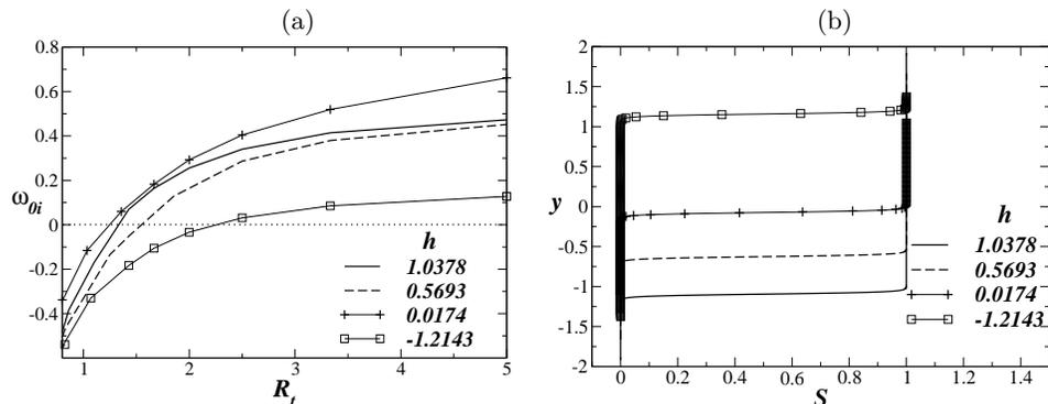
FIGURE 20. (a) Variation of  $\omega_{0i}$  with velocity ratio for different locations of the viscosity interface.  $R_s = -1$ ,  $\text{Re} = 100$ ,  $\text{Sc} = 1$ ,  $q = 0.1138$ . (b) The corresponding basic profiles of concentration  $S$ .
