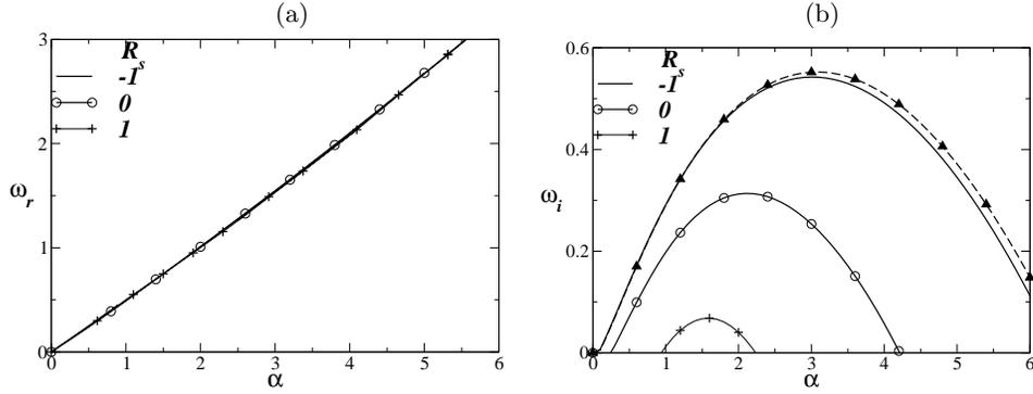
FIGURE 6. The dispersion curves (a)  $\omega_r$  versus  $\alpha$ , (b)  $\omega_i$  versus  $\alpha$  for different values of  $R_s$ . The dotted line with filled triangles represents dispersion curve for the base state obtained from the direct numerical simulation for  $R_s = -1$ . Values of the remaining parameters are  $Re = 100$ ,  $Sc = 1$ ,  $h = 0.569$ ,  $q = 0.1138$  and  $R_t[\equiv \Delta U/(U_\infty + U_{-\infty})] = 1$ .
