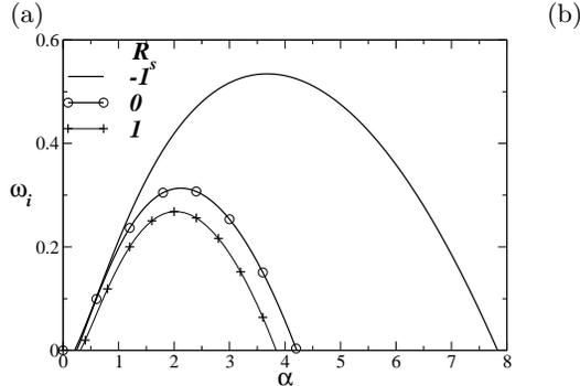
FIGURE 11. Dispersion curves for different values of  $R_s$  when  $h = 0$ , i.e., the centers of the two layers overlap. The remaining parameters are  $Sc = 1$ ,  $Re = 100$ ,  $q = 0.1138$  and  $R_t = 1$ .
