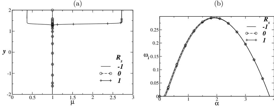
FIGURE 10. (a) Viscosity profile, (b) the dispersion curves  $\omega_i$  versus  $\alpha$ , for different values of  $R_s$ . Values of the remaining parameters are  $Re = 100$ ,  $Sc = 1$ ,  $h = -1.395$ ,  $q = 0.1138$  and  $R_t[\equiv \Delta U/(U_\infty + U_{-\infty})] = 1$ .
