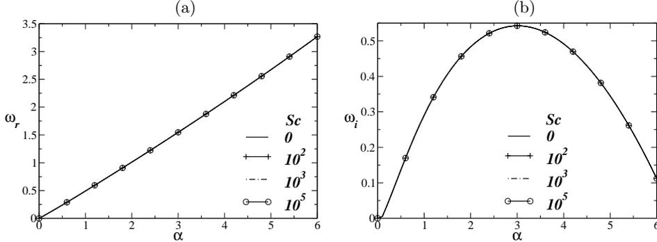
FIGURE 8. The dispersion curves (a)  $\omega_r$  versus  $\alpha$ , (b)  $\omega_i$  versus  $\alpha$  for different values of  $Sc$ . The other parameters are  $Re = 100$ ,  $h = 0.569$ ,  $q = 0.1138$ ,  $R_s = -1$  and  $R_t = 1$ .
