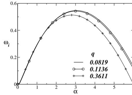
FIGURE 14. The dispersion curves ( $\omega_i$  versus  $\alpha$ ) for different values of  $q$ . Values of the remaining parameters are  $Re = 100$ ,  $Sc = 1$ ,  $h = 0.569$ , and  $R_t[\equiv \Delta U/(U_\infty + U_{-\infty})] = 1$ .
