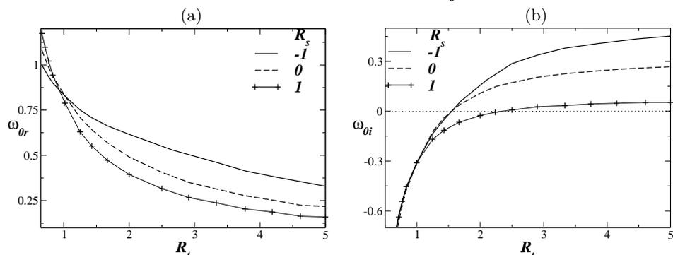
FIGURE 19. Frequency and growth rate of the zero group velocity mode, as a function of the velocity ratio, for three values of  $R_s$ . As before,  $\text{Re} = 100$ ,  $h = 0.5693$ ,  $q = 0.1138$ . Values of  $\omega_{0i} > 0$  indicate absolute instability.
