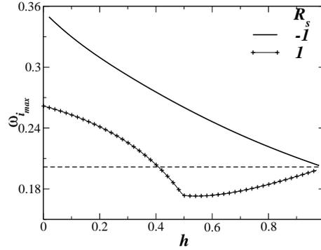
FIGURE 16. The dominant growth rate for the long wave mode as a function of the interface location  $h$ . The dashed line indicates the growth rate in the unstratified case. Given the symmetry in the problem, it is sufficient to consider only positive values of  $h$ .
