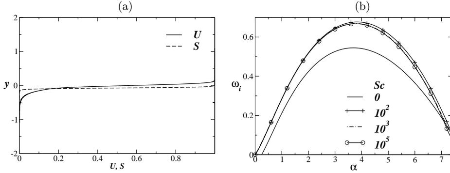
FIGURE 9. (a) The basic state velocity ( $U$ ) and concentration ( $S$ ) profiles; (b)  $\omega_i$  versus  $\alpha$  for different values of  $Sc$  for  $h = 0.0524$  (i.e. when the viscosity stratified layer overlaps with the momentum stratified layer). The other parameters are  $Re = 100$ ,  $q = 0.1382$ ,  $R_s = -1$  and  $R_t = 1$ .
