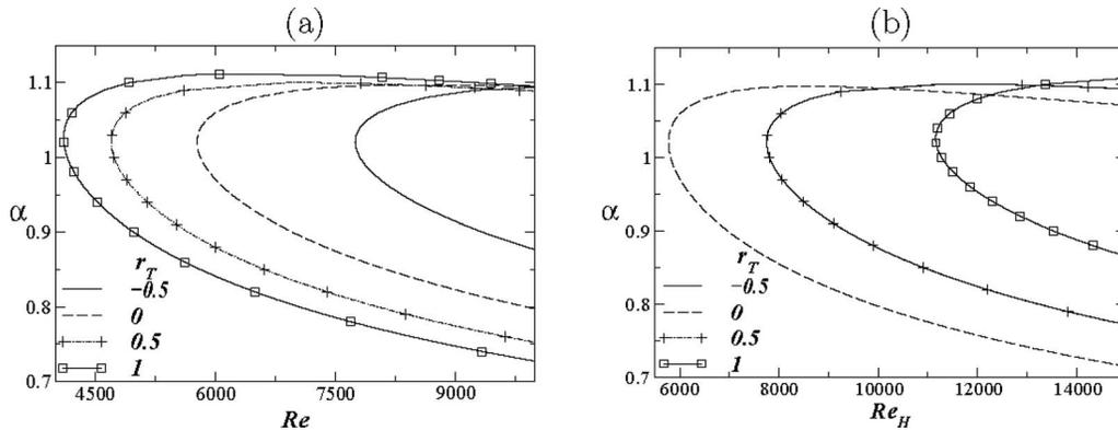
**Fig. 4** Stability boundaries for different values of  $r_T$ . The rest of the parameter values are  $Pr=0$ ,  $Gr=0$ , and  $Na=0$ . In Fig. 4(b),  $Re_H = U_m \rho H / \mu_{hot}$ . Note that the curves associated with  $r_T=-0.5$  and  $r_T=0.5$  in panel (b) are indistinguishable.
