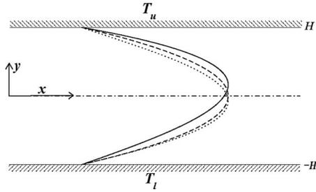
**Fig. 1** Schematic diagram of the channel; bottom and top walls are maintained at different, constant temperatures,  $T_l$  and  $T_u$ , respectively. Also shown here are profiles of the steady, horizontal velocity component generated with  $Na=0.86$ ,  $r_T=1$  (solid line),  $Na=0.86$ ,  $r_T=-0.5$  (dotted line), and  $Na=0$ ,  $r_T=0$  (dashed line).
