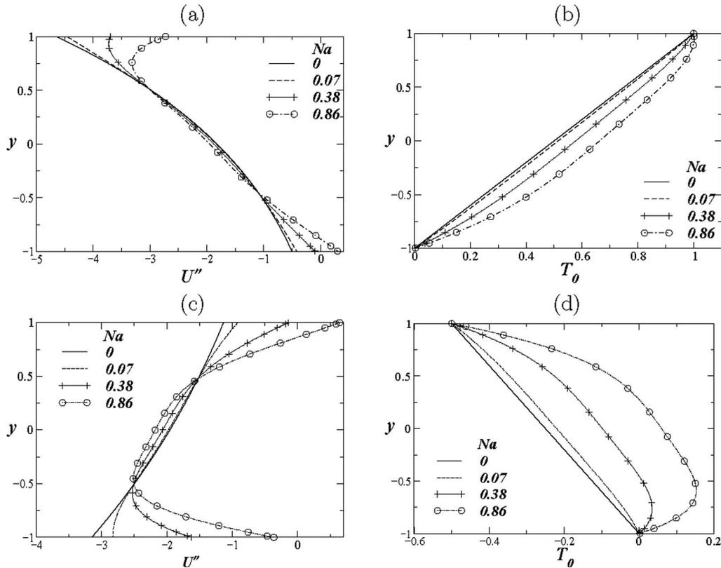
**Fig. 2 Basic state profiles of the second derivative of the horizontal component of the velocity ( $U''$ ) and temperature ( $T_0$ ) for different  $Na$  when  $r_T=1$  and  $r_T=-0.5$  are shown in (a) and (b) and (c) and (d), respectively**
