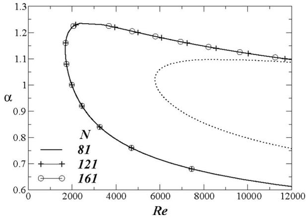
**Fig. 3** The effect of increasing the order of Chebyshev polynomials ( $N$ ) on the neutral stability curve with  $r_T=1$ ,  $Pr=1$ ,  $Gr=100$ , and  $Na=0.86$ . The dotted line shows the neutral stability curve for  $r_T=0$ ,  $Gr=0$ , and  $Na=0$ , which corresponds to isothermal flow through a channel; the critical Reynolds number for this case is 5772.2.
