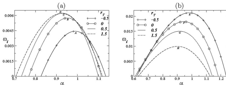
**Fig. 7 The effect of varying  $r_T$  on the dispersion curves for  $Na = 0.1$  (a) and  $Na = 1.1$  (b). The rest of the parameter values are the same as those used to generate Fig. 6. The labels A–H are used to designate the maxima in the dispersion curves; the energy budgets associated with these points are provided in Tables 3 and 4.**
