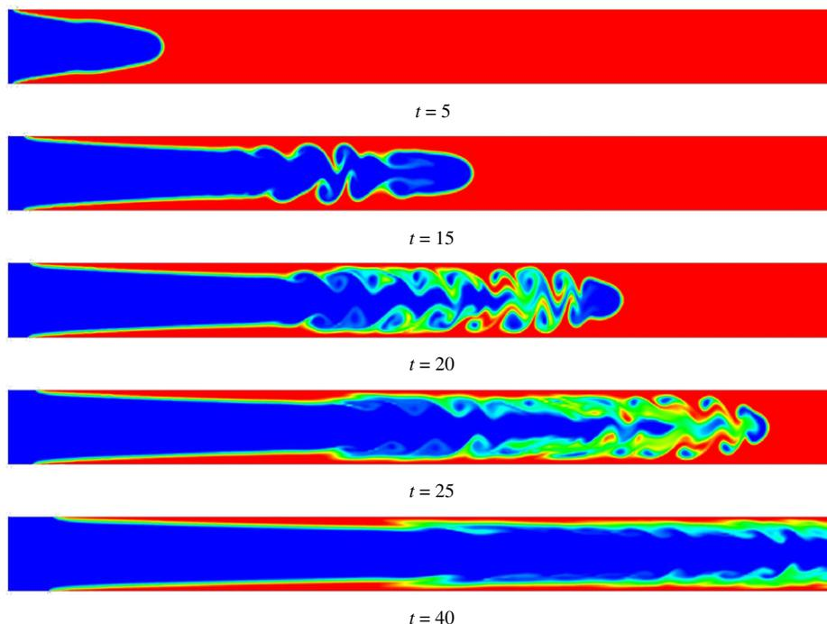
**Fig. 3.** Spatio-temporal evolution of the concentration contours for the isothermal ( $r_T=Na=0$ ). The rest of the parameter values are  $Re=500$ ,  $Sc=100$ ,  $Pr=7$ ,  $m=10$  and  $r_\kappa=1$ .
