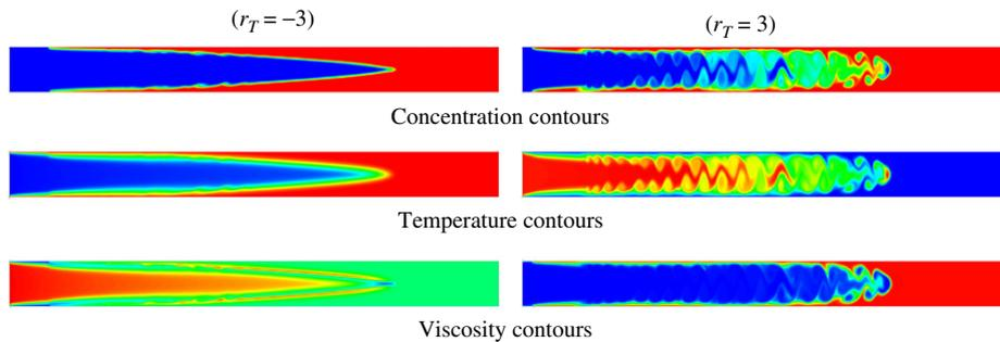
**Fig. 5.** The concentration, temperature and viscosity contours at  $t=20$  for  $r_T = -3$  and 3. The rest of the parameter values remain unchanged from those used to generate Fig. 3.
