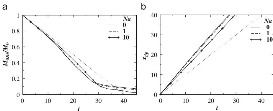
**Fig. 7.** The effect of  $Na$  on the mass fraction of the displaced fluid '1', (a), the temporal evolution of the position of the leading 'front' separating the two fluids  $x_{tip}$ , (b). The rest of the parameter values are  $Re=500$ ,  $Sc=100$ ,  $Pr=7$ ,  $m=10$ ,  $r_c=1$  and  $r_l=1$ . The dotted line in panel (a) is the analogue of those shown in Figs. 2a and 4a; and the dotted line in panel (b) is the analogue of those shown in Figs. 2b and 4b.
