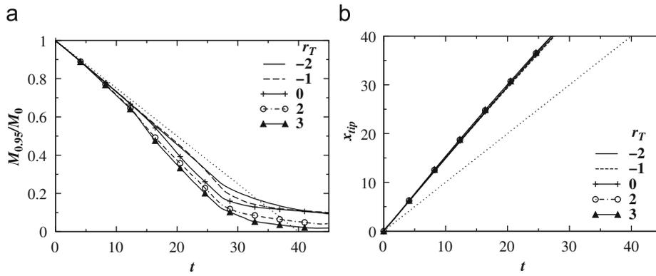
**Fig. 4.** The effect of  $r_T$  on the mass fraction of the displaced fluid '1', (a), the temporal evolution of the position of the leading 'front' separating the two fluids  $x_{tip}$ , (b), for  $Na=0$ . The rest of the parameter values are  $Re=500$ ,  $Sc=100$ ,  $Pr=7$ ,  $m=10$  and  $r_K=1$ . The dotted lines in panels (a) and (b) are the analogues of those shown in Fig. 2 a and b, respectively.
