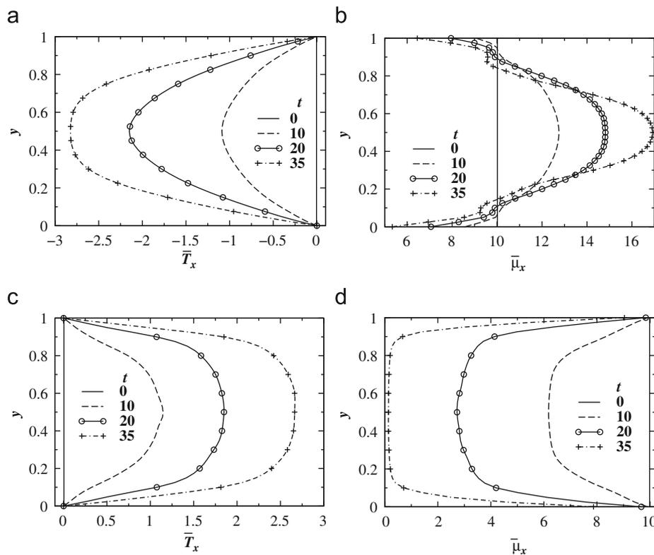
**Fig. 6.** Evolution of the transverse variation of the axial-averaged temperature ( $\bar{T}_x \equiv (1/L) \int_0^L T dx$ ) and viscosity ( $\bar{\mu}_x \equiv (1/L) \int_0^L \mu dx$ ) for  $r_l = -3$  and  $r_l = 3$  are shown in (a) and (b), and (c) and (d), respectively. The rest of the parameter values remain unchanged from those used to generate Fig. 3.
