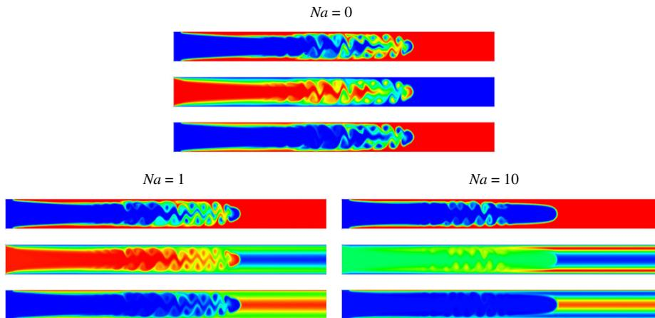
Fig. 8. The concentration, temperature and viscosity contours at  $t=20$  for different  $Na$  are shown in first, second and third panels, respectively. The rest of the parameter values remain unchanged from those used to generate Fig. 7.
