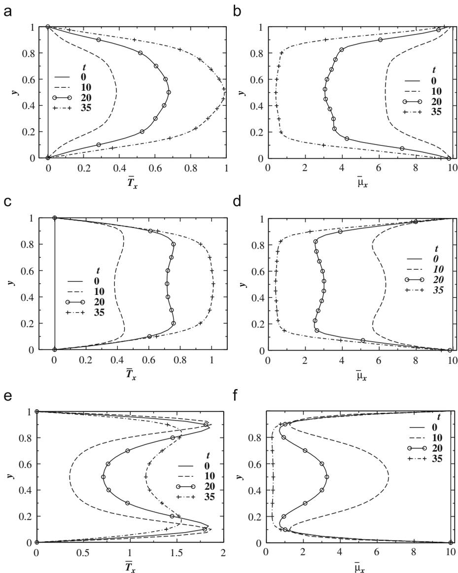
Fig. 9. Evolution of the transverse variation of the axial-averaged temperature ( $\bar{T}_x \equiv (1/L) \int_0^L T dx$ ) and viscosity ( $\bar{\mu}_x \equiv (1/L) \int_0^L \mu dx$ ) for  $Na=0, 1$  and  $10$  are shown in (a) and (b), and (c) and (d), and (e) and (f), respectively. The rest of the parameter values remain unchanged from those used to generate Fig. 7.
