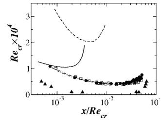
**Fig. 4 Axial variation of the critical Reynolds number. Filled triangles, axisymmetric mode at  $r=0.25$ . Filled circles and open squares, experimental results [13]. The theoretical results of Refs. [18,19] for axisymmetric disturbances are shown by the dashed and solid lines, respectively. The results of Refs. [13,18,19] were compiled in this manner in Ref. [15].**
