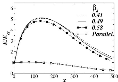
**Fig. 3 Amplification of the disturbance kinetic energy for the axisymmetric ( $n=0$ ) mode for typical disturbance frequencies for  $Re=5000$  at  $r=0.08$ . The result with a parallel flow assumption is shown by the solid line with squares.**
