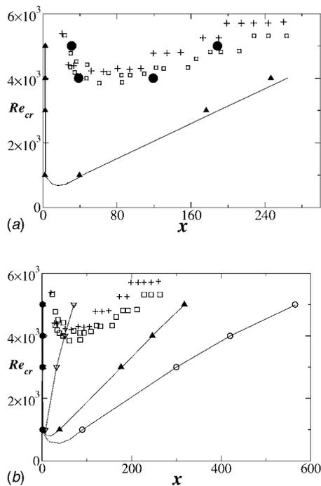
**Fig. 5 Axial variation of the critical Reynolds number ( $n=0$  mode). Plus and open squares: experimental results [13] for nonaxisymmetric and axisymmetric disturbances, respectively. (a) At  $r=0.25$ . Filled triangles, neutral boundary; filled circles, where  $E/E_{cr}=1.8$ . (b) Open circles,  $r=0.5$ ; filled triangles,  $r=0.25$ ; open triangles,  $r=0.08$ . The lines are shown to guide the eye.**
