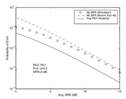
Fig. 1. Error performance as a function of average SNR for  $K=2, M=2, \ N=1, \ {\rm NFR}=0 \ {\rm dB}.$
