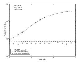
Fig. 2. Bit error performance as a function of NFR. K=2, M=2, N=1, SNR=10 dB.
