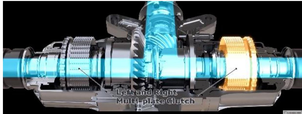
Application of clutch plates with hydraulic actuators to
