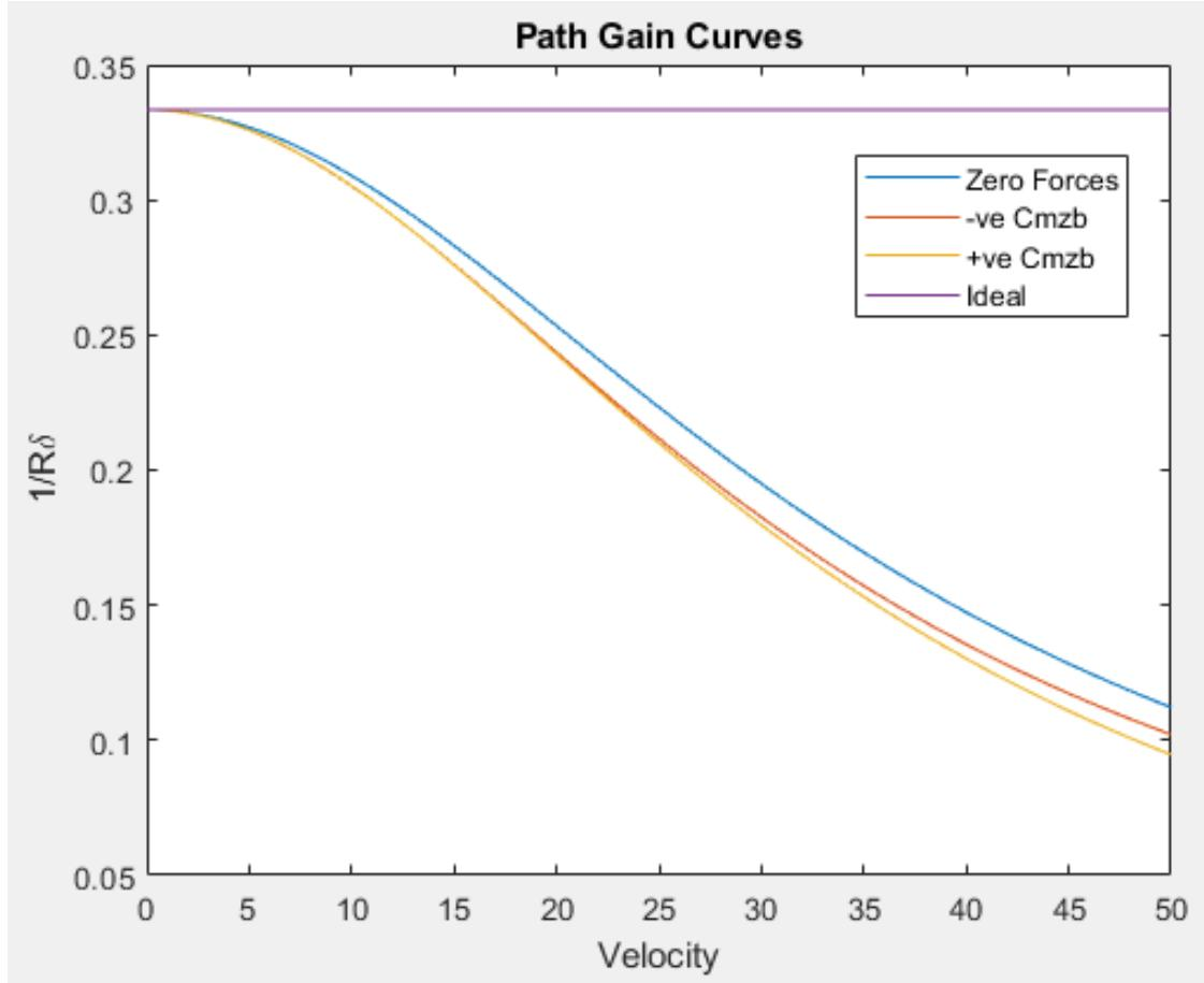
The path gains were plotted for the condition with no aerodynamic forces and aligning torques, Condition with positive  $C_{mz,\beta}$  and also for the Condition with negative  $C_{mz,\beta}$  and finally the ideal kinematic path gain has also been plotted for a Car track length of 3 m.
