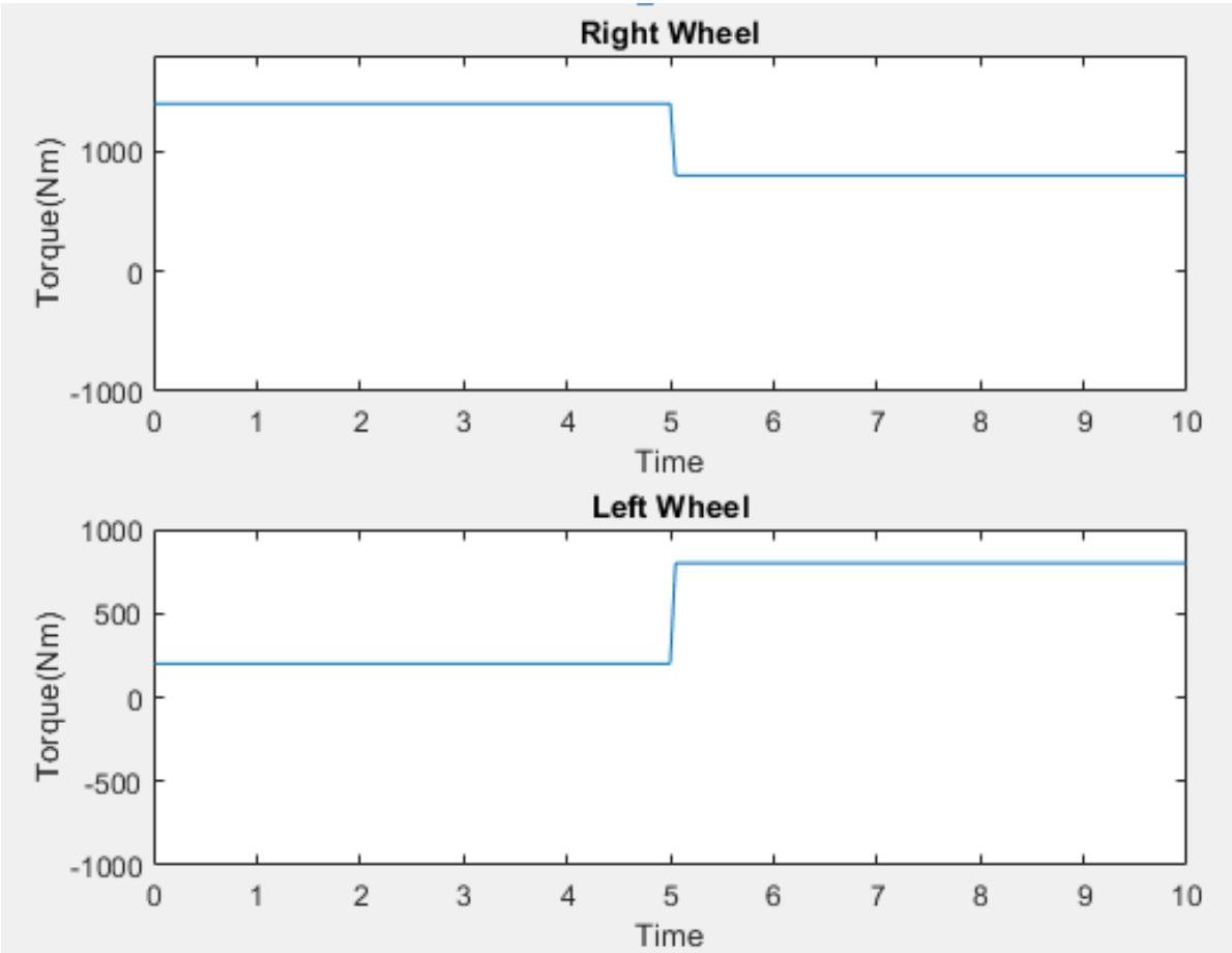
Required Yaw moment converted to Torque :
