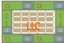
A Chipmultiprocessor (CMP) with non-tiled architecture.
