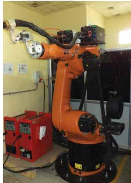
Robotic Welding Machine Twin-Wire
