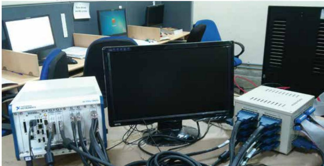
NI-PXIe-1062Q with Interface Module
