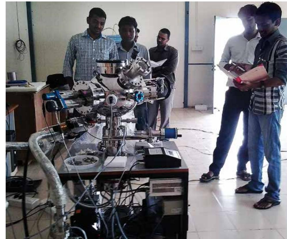
Pulsed laser deposition set up
