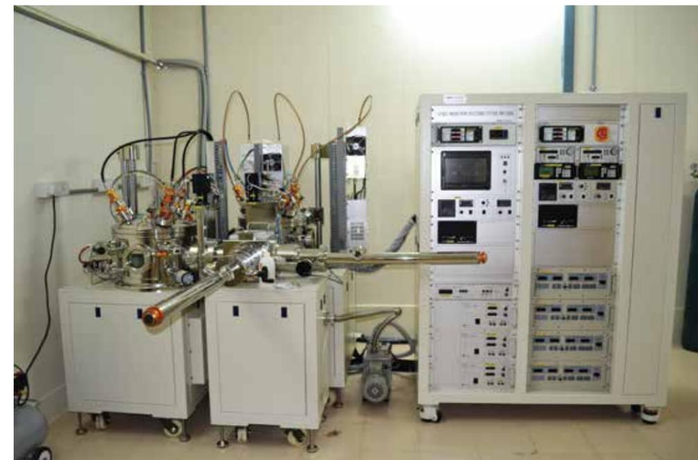
RF & DC Magnetron Sputtering
