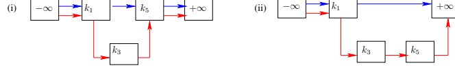
Fig. 9: Delete of k_5 in STM\_tryC() . k_5 is unlinked from bl by linking bl of k_1 to \infty .
