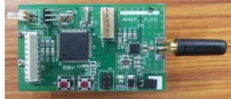
Fig. 5: IITH Mote used for test bed deployment
