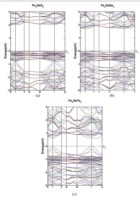
Figure 2. Calculated band structure of (a) Fe<sub>2</sub>GeS<sub>4</sub>, (b) Fe<sub>2</sub>GeSe<sub>4</sub> and (c) Fe<sub>2</sub>GeTe<sub>4</sub>.
