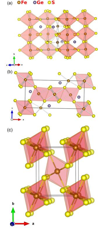
**Figure 1.** Crystal structure of (a) edge-sharing octahedra and (b) vertex-sharing octahedra of  $Fe_2GeS_4$  compared with (c) marcasite  $FeS_2$ .
