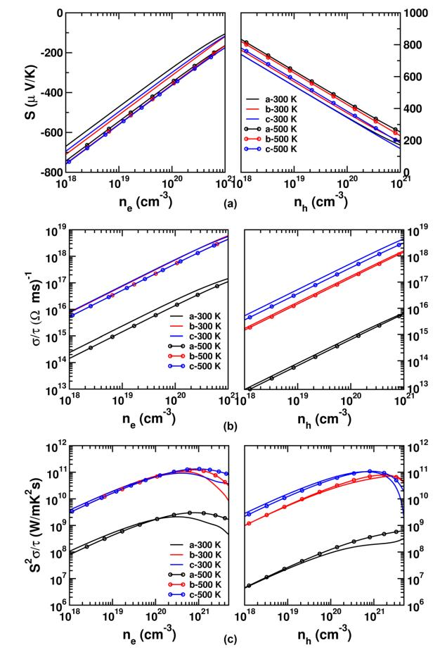
Figure 7. Calculated (a) thermopower, (b) electrical conductivity scaled by relaxation time and (c) power factor for Fe<sub>2</sub>GeSe<sub>4</sub>.
