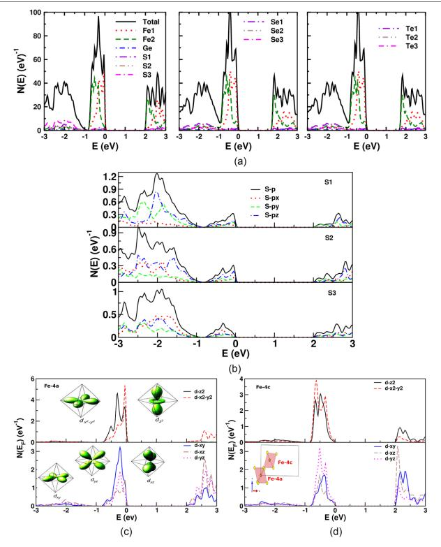
Figure 4. (a) Calculated DOS of Fe<sub>2</sub>GeCh<sub>4</sub>, and *m*-projected DOS for (b) S-*p*, (c) Fe1 at 4*a* and (d) Fe2 at 4*c* positions of Fe<sub>2</sub>GeS<sub>4</sub>.
