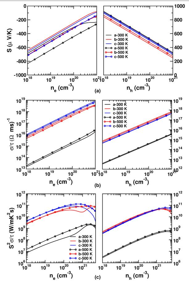
Figure 6. Calculated (a) thermopower, (b) electrical conductivity scaled by relaxation time and (c) power factor for Fe<sub>2</sub>GeS<sub>4</sub>.
