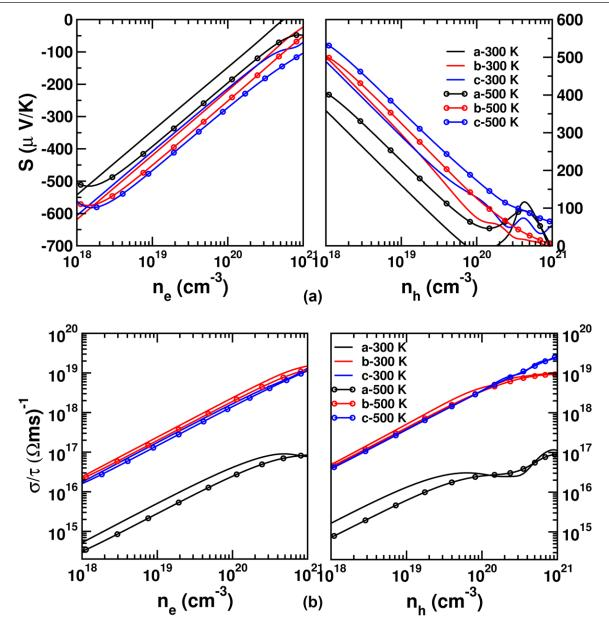
Figure 8. Calculated (a) thermopower and (b) electrical conductivity scaled by relaxation time for Fe<sub>2</sub>GeTe<sub>4</sub>.
