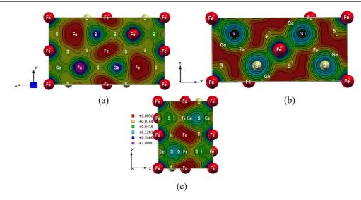
**Figure 5.** Calculated charge density density along the (a) xy, (b) xz and (c) yz planes of Fe<sub>2</sub>GeS<sub>4</sub>.
