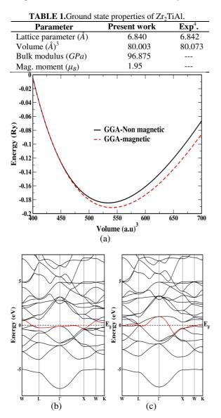
**FIGURE 1.** Energy optimization (a), band structure for spin-up (b) and spin-down (c).
