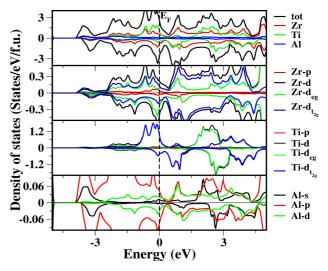
FIGURE 3. Density of states for Zr<sub>2</sub>TiAl.
