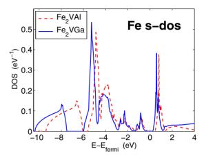
FIG. 3. (Color online) Calculated Fe 4s partial density of states (in units of electrons per eV and per Fe atom) in Fe<sub>2</sub>VAl (dashed and red) and Fe<sub>2</sub>VGa (full line and blue). The zero of energy is placed at the Fermi level, which falls in the pseudo gap within the Fe and V d bands. The full density of states for these compounds have been discussed in Refs. 12–14.
