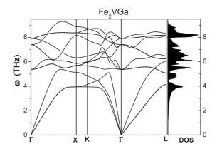
FIG. 2. Calculated phonon dispersion curves and phonon density of states of Fe<sub>2</sub>VGa
