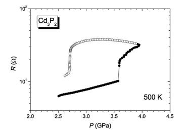
Fig. 7. Pressure dependence of the electrical resistance of a  $Cd_3P_2$  sample at 500 K. The notation is as in Fig. 2.
