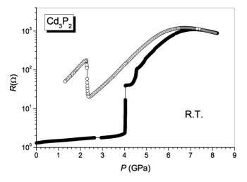
Fig. 2. Pressure dependence of the electrical resistance of a  $Cd_3P_2$  sample at room temperature. Filled circles denote compression, and open circles decompression. Note the phase transformation at 4.0 GPa upon compression and the hysteresis in decompression.
