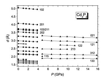
Fig. 5. The observed lattice plane spacing, d, are shown as a function of pressure. Filled circles denote the tetragonal phase, and filled triangles the orthorhombic phase. For clarity, indices hkl are shown only for the first five lines of the tetragonal phase. The full lines are guides for the eye.
