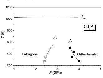
Fig. 9. P-T diagram of phase transitions in Cd<sub>3</sub>P<sub>2</sub>, observed by resistance measurements. Solid symbols denote compression, and open symbols decompression. Triangles denote regions, where a metastable phase is formed. The solid line is the melting curve of Cd<sub>3</sub>P<sub>2</sub> [2].
