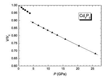
Fig. 6. Experimental compression curves of Cd<sub>3</sub>P<sub>2</sub>. The notation is as in Fig. 5. The relative volume change at the tetragonal to orthorhombic transition is  $\Delta V/V = -5.5\%$ .
