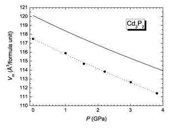
Fig. 4. Compression of tetragonal  $Cd_3P_2$  at room temperature. The dashed curve through the experimental data points has been calculated from the Birch–Murnaghan equation (1). The result of the theoretical calculation is shown by the full curve.
