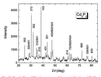
Fig. 10. Powder X-ray diffraction spectrum of the metastable phase of Cd<sub>3</sub>P<sub>2</sub> at ambient conditions. The wavelength of the X-rays is  $\lambda = 1.54056$  Å (Cu K $\alpha_1$ ). The metastable phase was obtained by heating the sample to 720 K at 3.6 GPa. For clarity, indices are shown only for major reflections (cf. Table 1, where all reflections are indexed).
