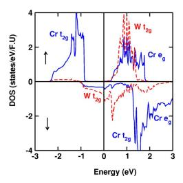
FIG. 1. (Color online) Orbital resolved density of states (DOS) of Sr<sub>2</sub>CrWO<sub>6</sub> with spin-orbit coupling. The Fermi energy is indicated by zero energy level.
