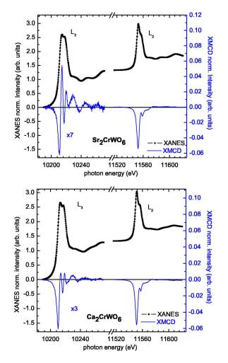
FIG. 2. (Color online) XANES spectra and derived XMCD spectra for  $Sr_2CrWO_6$  (upper panel) and  $Ca_2CrWO_6$  (lower panel). The XANES spectra (symbols) are corrected as described in the text. The XMCD spectra are shown as full lines. The XMCD spectrum of the W  $L_3$  edge was multiplied by a factor of 7 for  $Sr_2CrWO_6$  and by a factor of 3 for  $Ca_2CrWO_6$  for clarity.
