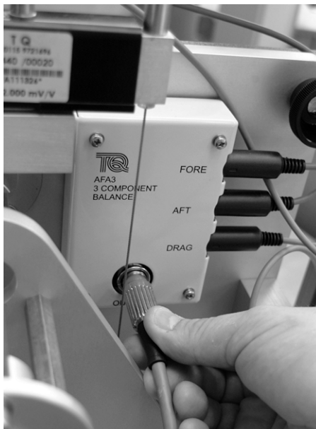
Figure 5 Use the 7 pin DIN type Lead to Connect the Balance to the Display Module
