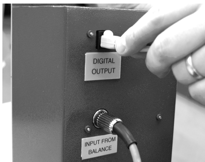
Figure 6 Use the Cable Supplied with the VDAS To Connect up the AFA3 Display Module
