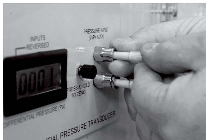
Figure 7 Push and hold the pressure socket to remove the pipe connection
