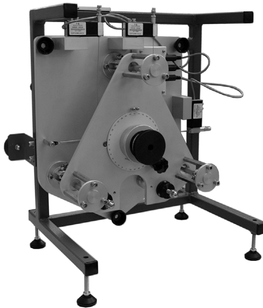
Figure 12 The AFA3 Three Component Balance on its calibration/storage frame.
