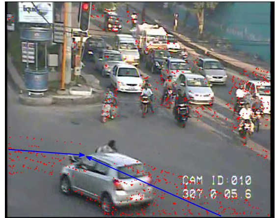
Fig. 5. The intersection of two trajectories during an accident. The trajectories of the motorcycle and car intersect each other also there is no further progress in the trajectories of the motorcycle and car, thus considered as a collision.
