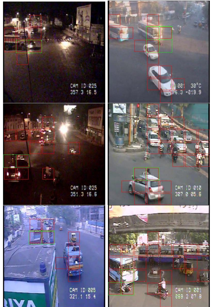
Fig. 11. Accident detected using proposed approach for different videos. The red region is the predicted accident regions using a single score either by appearance, motion, or intersection of tracks while the green box shows the region decided using final score. [Best viewed in color]
