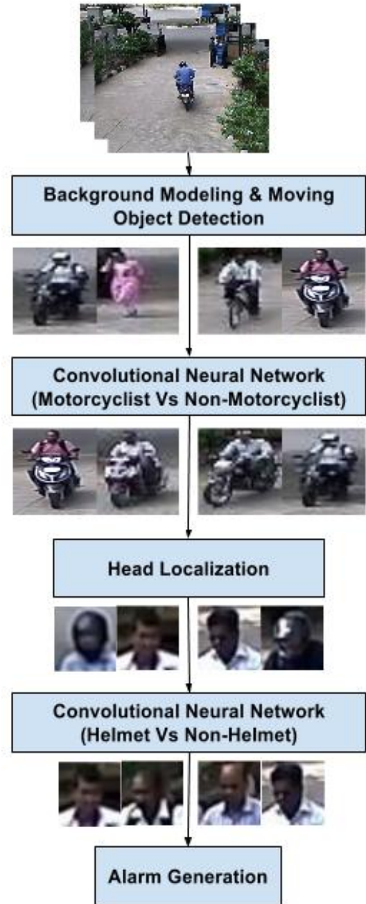
Fig. 1. Block diagram of proposed framework for the detection of motorcyclists without Helmet
