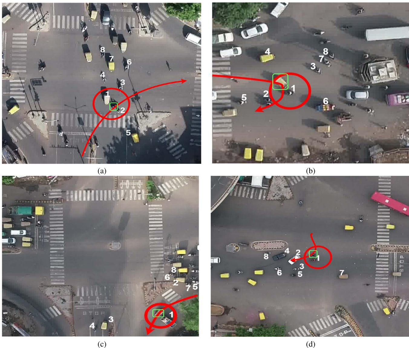
Fig. 4. Examples of unsafe interaction trajectories in SkyEye dataset at various intersections - (a) P, (b) A, (c) N, and (d) V. The vehicle whose interaction trajectory is under consideration is shown in green and its neighbors for that particular instant are shown with numbers in white. The trajectory is shown in red and an unsafe interaction is marked in red.
